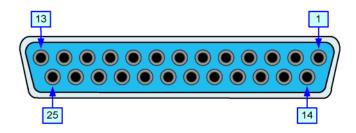
Figure 3-5, Serial Connector Pin Assignments
